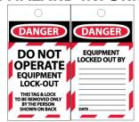
Attach a "Do Not Operate" warning tag to the start switch or controls before the equipment is serviced or repaired. Attach the warning tags to the engine and to each operator control panel. When appropriate disconnect the negative terminal on the battery.
